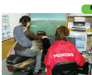
▲ Motorcycle riding simulator You need to have a motorcycle license to get on this simulator. It tests your ability to perform both ordinary braking and emergency braking as another car jumps out from a cross street, and a professional rider instructs you on braking technique and timing.
