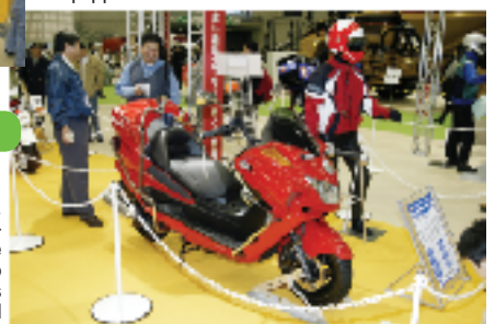
► Mist Dragon A fire-fighting motorcycle. Equipped with a high-pressure tank, this motorcycle can spray enough mist to extinguish two car fires. This is popular with children and adults alike.
