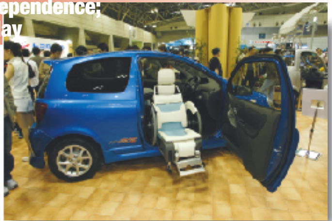
▲Toyota Auto Body has a vehicle that can be driven while still in your wheelchair.
