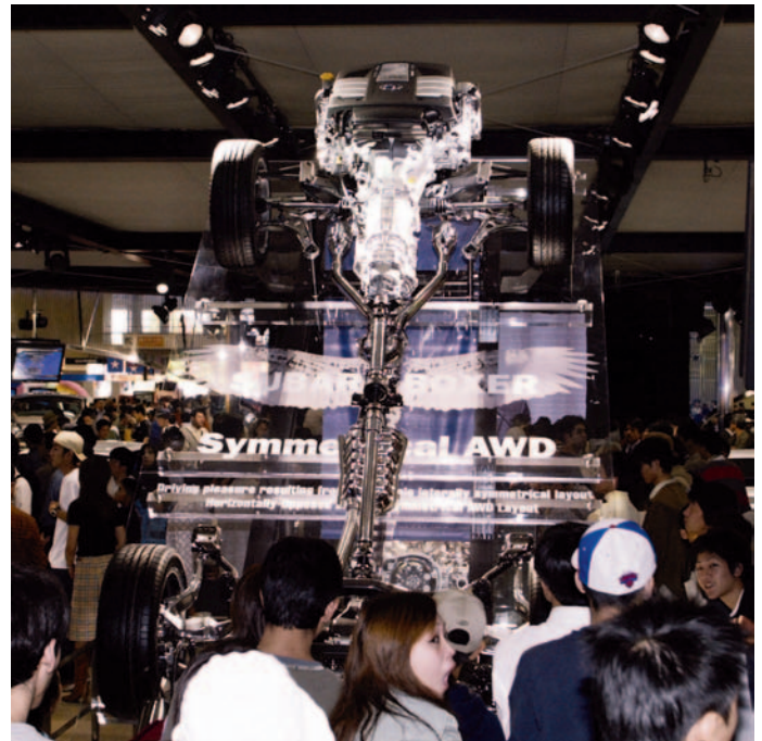
A cutaway model and the new horizontally opposed engine in the technology corner.
